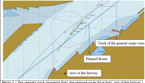
Photo 1 – The vessel's track (magenta line), the planned route (blue line), axis of the fairway (dashed black line) in the vicinity of the place of collision.
